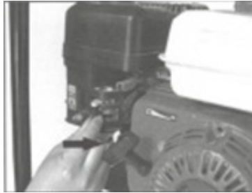
Open the fuel valve to the "ON" position
